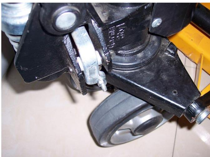
1. Loosen the setting screw (140H) on the crank link (139H).
