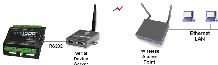
COM1000 connected to a wireless serial device server
