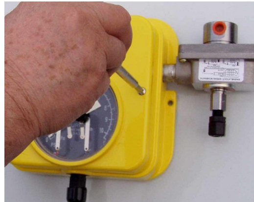
Fig. 11 Cover is to be closed and secured with front screws to insure proper sealing and protection from environment .
