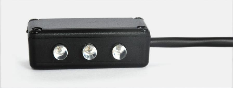
The control unit GRIPone is designed for connecting the Remotcontrol, a device that enables the display of control activity. The Remotcontrol, once connected and positioned so as to be visible while driving, inform the pilot when the traction control system comes into operation. At any time the GRIPone reduce the engine power the three led of Remotcontrol is switched on.
