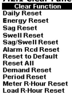
Clear function was designed to allow user to easily move and/or reset different data stored in this instrument.
