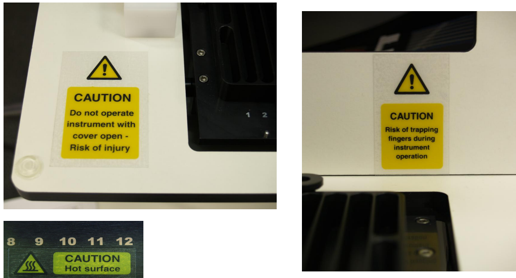
Fig.3: Warning Labels on B20
