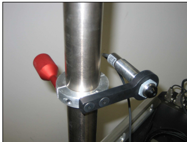
Figure 5.4: IR Temp. Sensor Installed on Column
