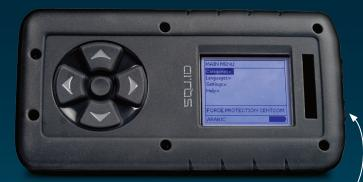
RESET Button: In the unlikely event of a lockup, your RESET button is located within your DC-In Port at the base of the unit (labeled "10-18VDC" on device)
