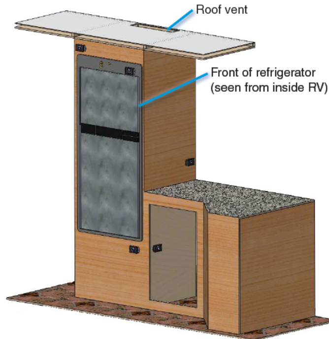
Fig. 3 Typical Inside View of Refrigerator Installation
