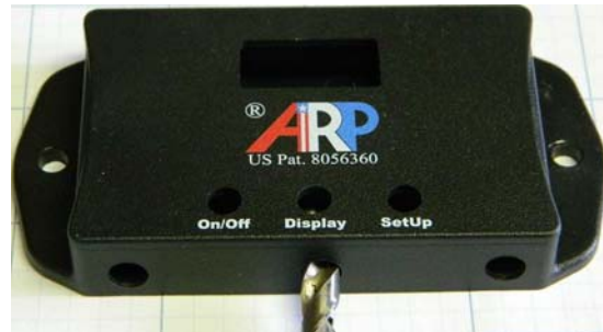
Fig. 9 Drill Drain/Wire Routing Holes
