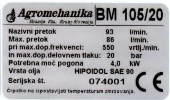
Sample of an identification plate on a pump
