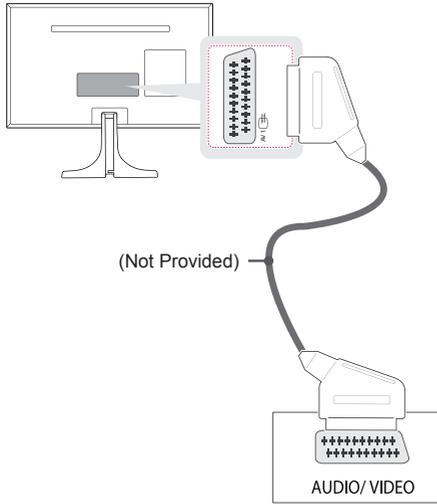
Transmits the video and audio signals from an external device to the TV set. Connect the external device and the TV set with the euro scart cable as shown.
