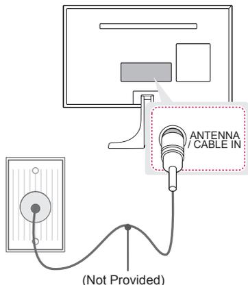
Connect the TV to a wall antenna socket with an RF cable (75 Ω).
