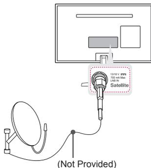
Connect the TV to a satellite dish to a satellite socket with a satellite RF cable (75 Ω).
