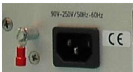
ground connector and main power socket
