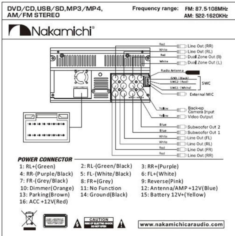
**NOTE:** Never connect cable to the system while it is connected to the battery power. Whenever the unit is disconnected from the battery, the preset memory will be erased and the unit will go back to its factory defaults.
