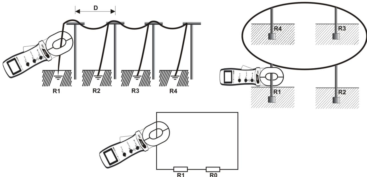
Fig. 9: Instrument's connection to a multiple-rod system
