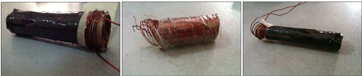
Figure 19: Eddy Current Probes (hand wounded)
