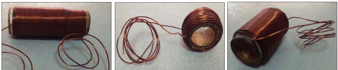
Figure 26: Eddy Current Probes (machine wound)
