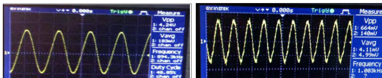
Figure 23: OPA564 Howland results (Resistive & Inductive loads)
