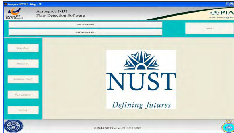
Figure 4: ET GUI Figure with buttons disabled until input files are selected
