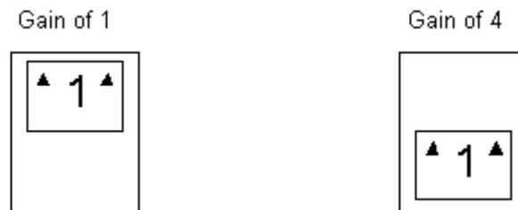
Figure 14 – Gain Switch Settings
