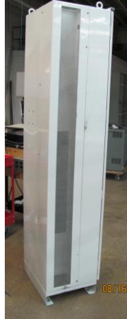
Figure 16: DRI-10 Side view showing ventilation louvers.
