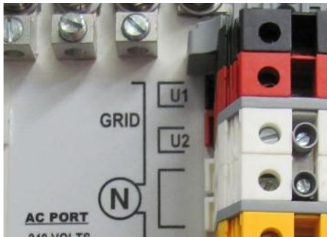
Figure 23: Grid port wiring connections.
