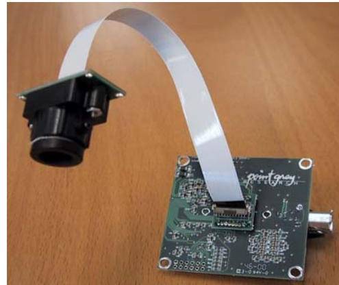
Figure 17: Assembled extended head camera
