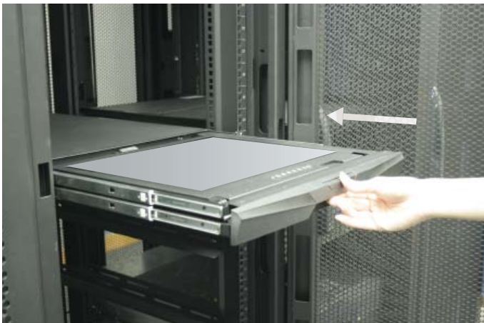
Figure 6. Slide the LCD keyboard drawer by pressing the carry handle button.
