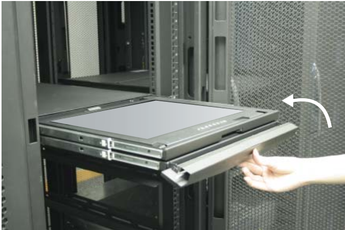
Figure 5. Flip up the front panel.
