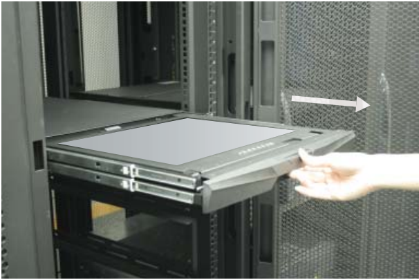
Figure 1. Pull the LCD drawer out of the rack.
