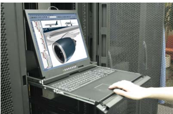
Figure 4. Operating the LCD keyboard drawer.
