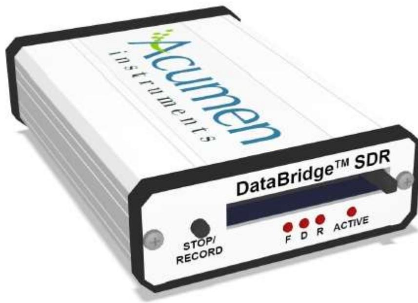
1. "Active" LED should be on when power applied
