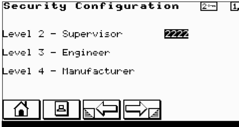
This screen can only be selected by the current level 4 password holder. Enter or reassign the password level codes.
