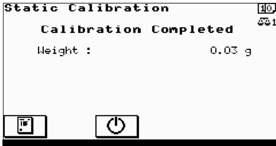
6. Check successful calibration by displayed weight agreeing with actual weight on weigher.
