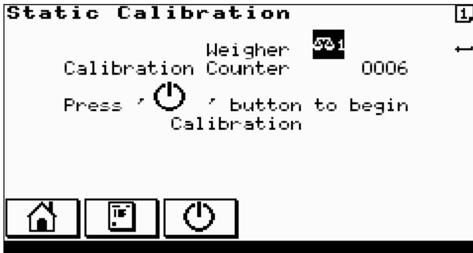
1. Before commencing for multi-weigher machines select the weigher to calibrate with the ENTER key. The **Calibration Counter** displayed on this first screen is a non-resettable counter that increments after each successful calibration. It is a weights and measures requirement to ensure no unauthorised calibrations can be performed.
