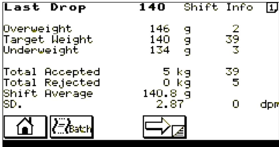
Shows weights, occurrences and standard deviation for batch and shift statistics. Use batch/shift button to move between the two statistics sets. See section 0
