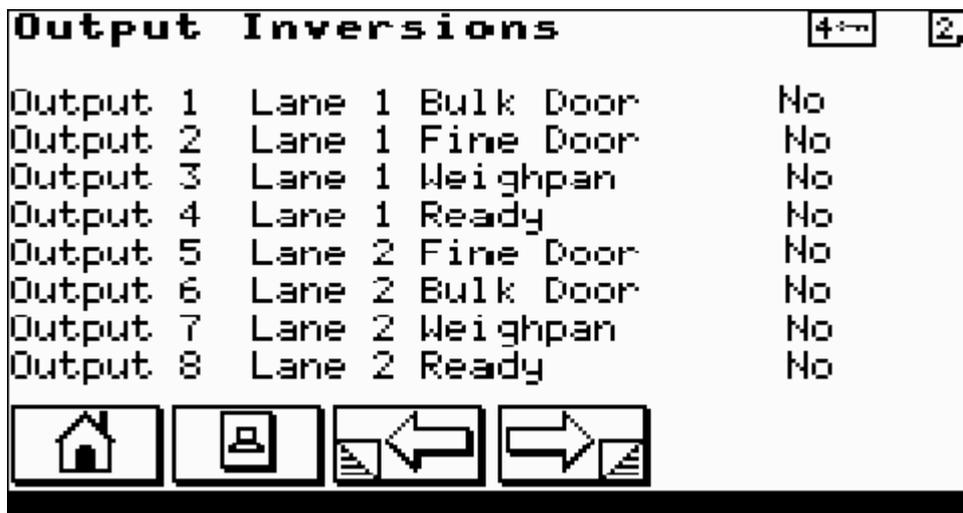
This screen allows the sense of each individual digital output to be inverted. Use the ENTER key to toggle between YES/NO.
