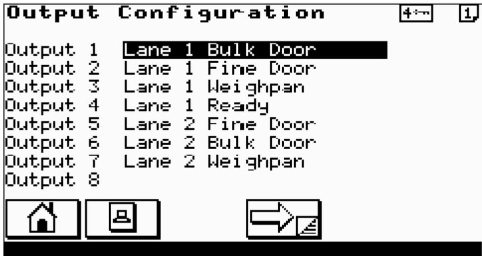
This screen allows each digital logical output to be assigned to a physical output. Use the ENTER key to select the logical output and the UP/DOWN ARROW keys to select the physical output.
