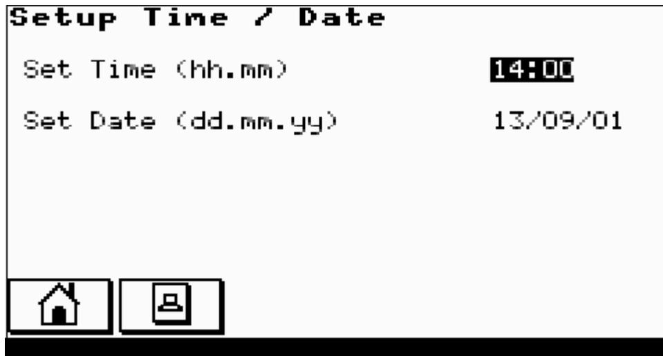
Setup current time and date. The system clock is battery backed and will maintain the correct time even when the machine is switched off.
