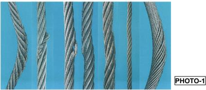
1) Loose, kinked, crushed, bird caged wire rope, waviness (more than 4/3d) or any damage resulting in distortion of the rope structure.
