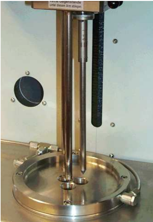
Triple bore capillary rheometer with thermal conductivity probe
