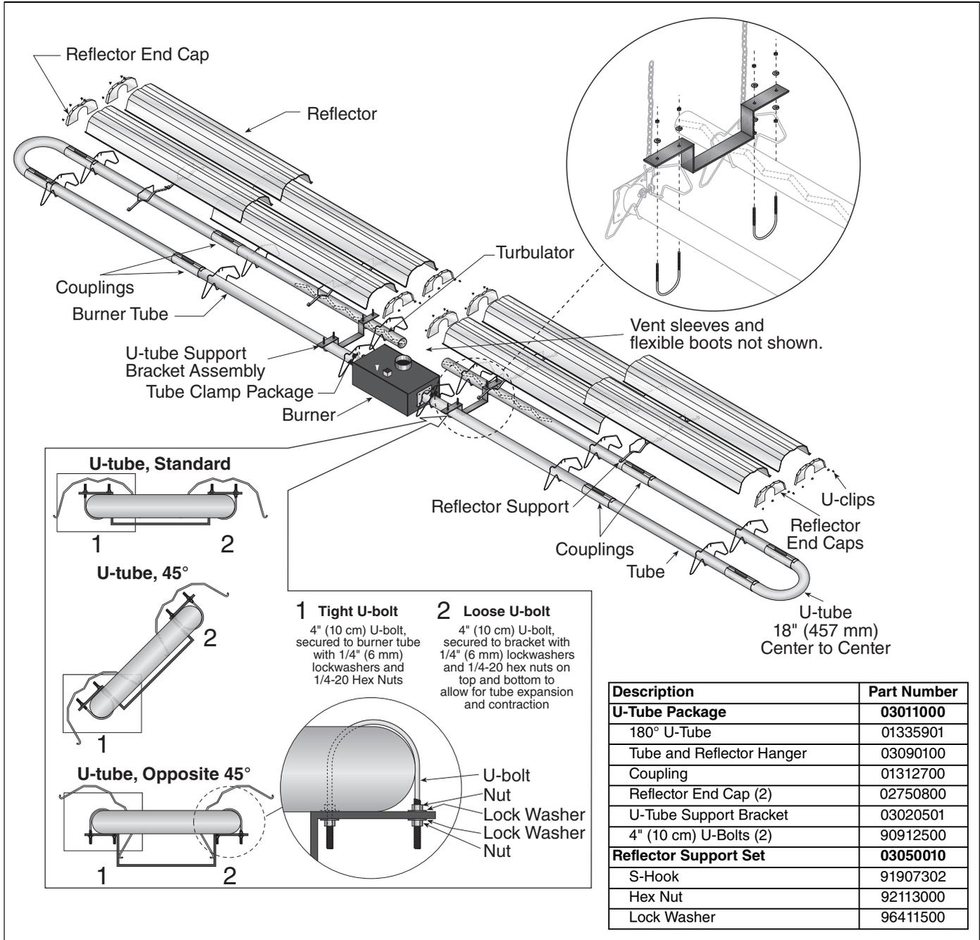
**FIGURE 19: U-Tube Heater Layout Overview**
