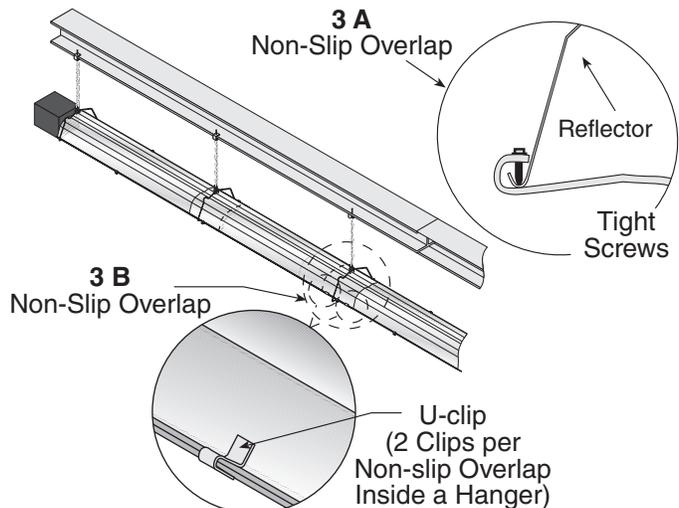
This section of three reflectors joined together must be affixed to the tube with at least one reflector support with tight screws.
