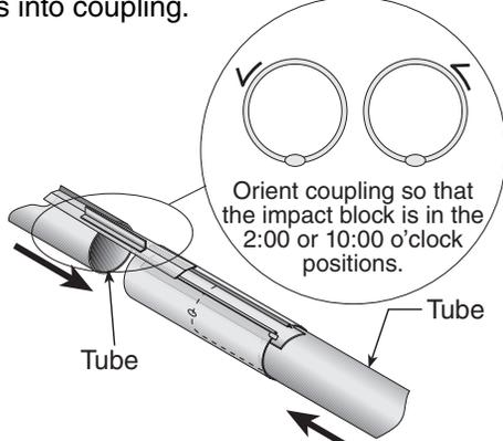
Orient coupling so that the impact block is in the 2:00 or 10:00 o'clock positions.
