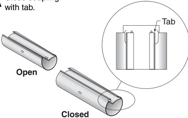
**B** Start Slide bar/Coupling Lock onto coupling.
