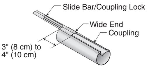
**C** Insert tubes into coupling.
