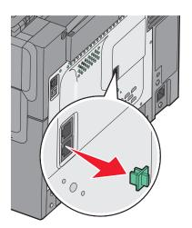
**2** Connect your telecommunications equipment directly to the bottom EXT port  $\widehat{}$  on the back of the printer.
