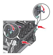
**16** Rotate the blue levers down until the imaging kit drops into place.
