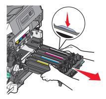
Remove the used developer unit.
