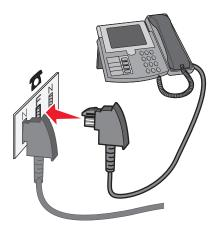
4 If you would like to use the same line for recording messages on your answering machine, then connect a second telephone line (not provided) between the answering machine and the other N slot of the active analog telephone wall jack.
