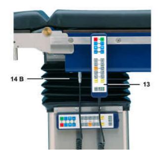
The control unit **13** is connected via the spiral cable to the connection socket on the left hand side (on the side with the column control panel) below the operating table top frame of the central section.
