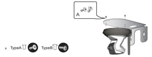
2. Fix the bracket and camera to the ceiling using the two screws and hollow wall anchors.
