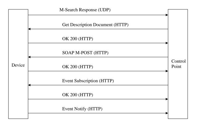
Figure 2: UPnP client server unicast communication
