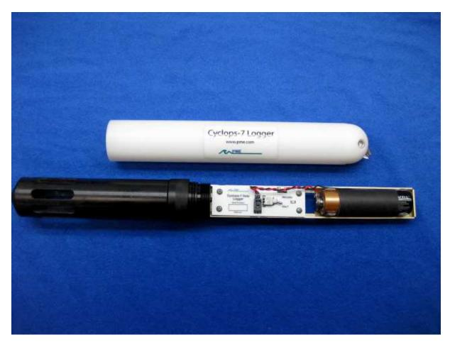
The logger circuitry is contained in a waterproof housing that must be opened. The housing is opened by unscrewing the white pressure housing from the black end cap. Turn the pressure housing counter clockwise relative to black end cap. Close by reversing this procedure after being sure that the o-ring is free from debris. Lube o-ring occasionally with grease intended for buna-n o-ring material.
