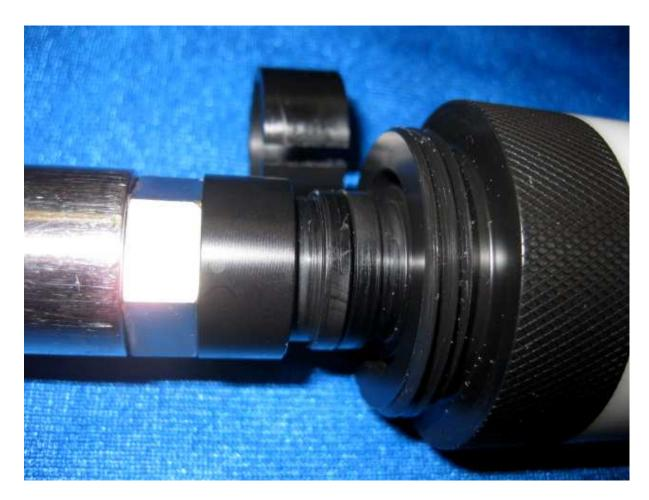
The clip faces will mate. Note that if the clip is not fully screwed onto the connector it will still appear as shown in the picture above, but the sensor may not be making complete reliable contact with the logger.
