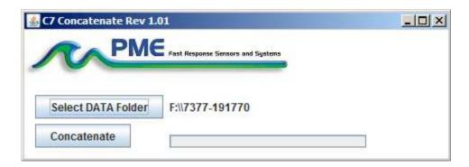
Cyc7Concatenate concatenates the files recorded by the Cyclops-7 Logger. The software reads all Logger files in a folder, except the CAT.txt file. Software translates Logger time stamps into two additional formats, and saves the result in a CAT.txt file in the DATA Folder.
