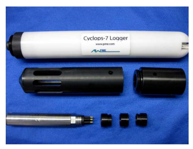
The small circular black clip shown to the right of the C7 sensor will be found installed on the logger connector. This can be removed by unscrewing it from the connector, and then gently prying open the 'C' clip center piece.
