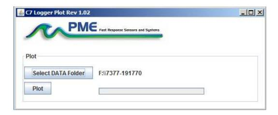
C7Plot plots the files recorded by the Cyclops-7 Logger. The software reads all Logger files in a folder, except the CAT.txt file.
