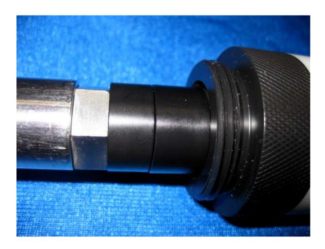
Slide the sensor support (middle-right in first picture) over the sensor. Note this part has an internal o-ring that comes against the sensor. This is not a water-proof seal. It's purpose is to firmly secure the sensor within the support. Next screw the sensor guard (middle left in first picture) onto the sensor support. The completed assembly is shown in the picture below.
