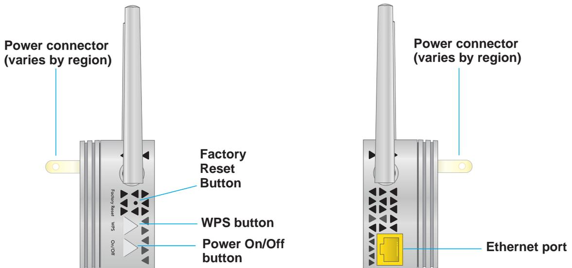
Figure 2. Buttons and port on the side panels
