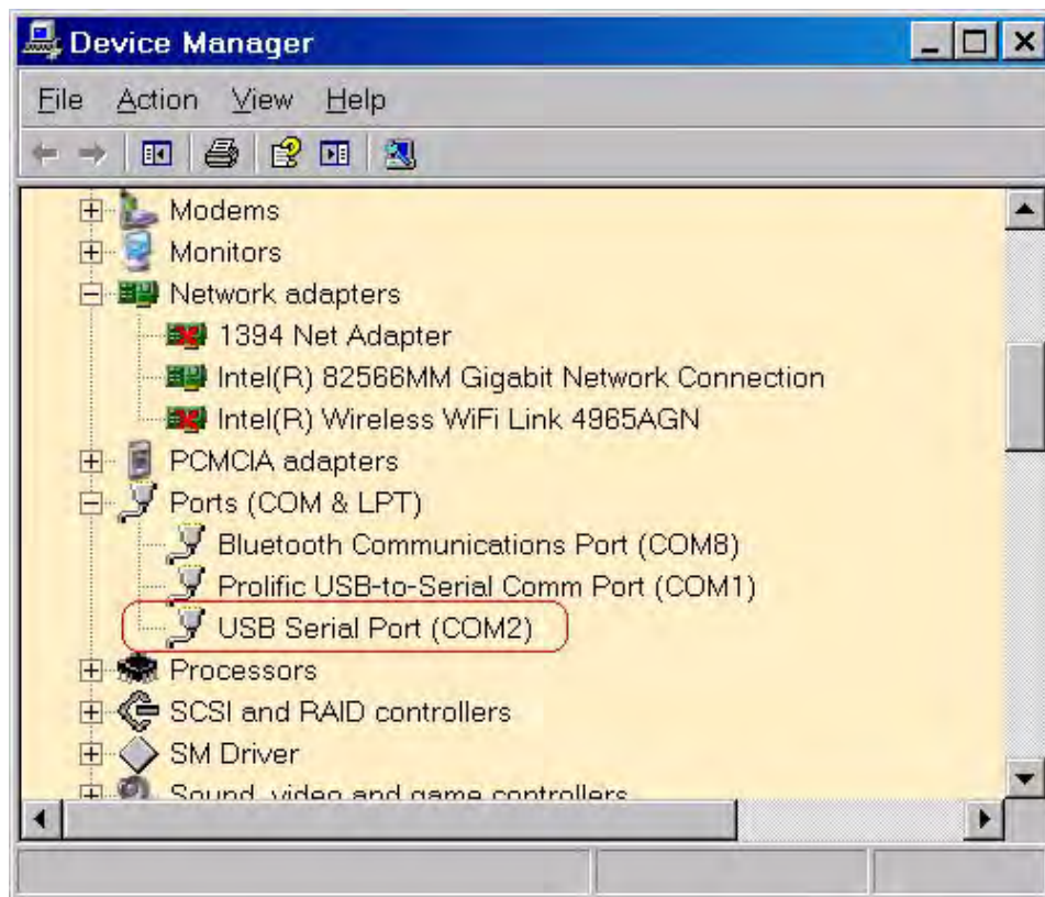
Figure 11. A Successful USB-to-UART Driver Installation
