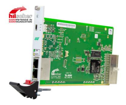
The F752 is based on the netX SOC. This highly integrated network controller supports parallel data transmission via several data paths between the internal CPU and graphics engines, and the communication and host controllers. The netX SOC also controls the on-board memory and other peripheral interfaces such as UARTS, USB, SPI or I<sup>2</sup>C.
