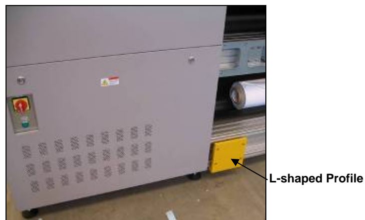
Figure 2. L-shaped Profile for Shipping Support
