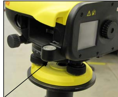
The Theodolite's Leveling Bubble
