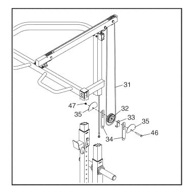
Do not overtighten the cables. If the cables are overtightened, the weight carriage will lift away from the base of the weight bench. If a cable tends to slip off the pulleys often, it may have become twisted. Remove the cable and reinstall it. If the cables need to be replaced, see the part ordering information on the back cover of this manual.
