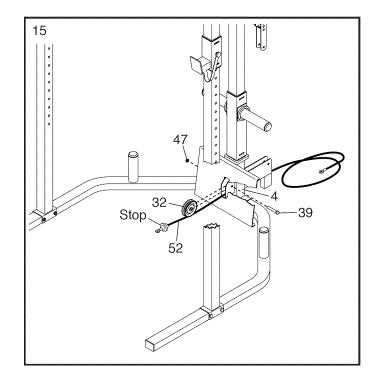
16. Insert a Pulley (32) over the Long Cable (52) inside the Guide (4). Attach the Pulley with an M10 x 45mm Bolt (39) and an M10 Locknut (47).
