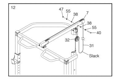
13. Insert a Pulley (32) into the loop of the Short Cable (31) as shown.
