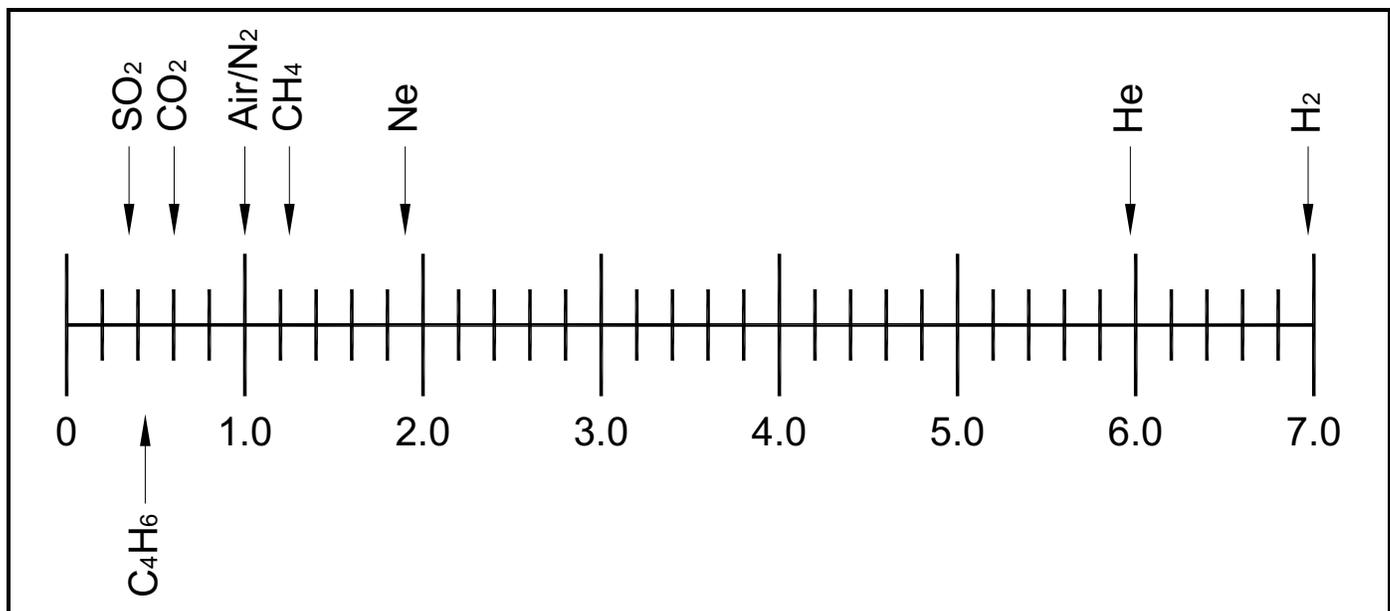
Figure 1: Relative Thermal Conductivity of Some Common Gases
