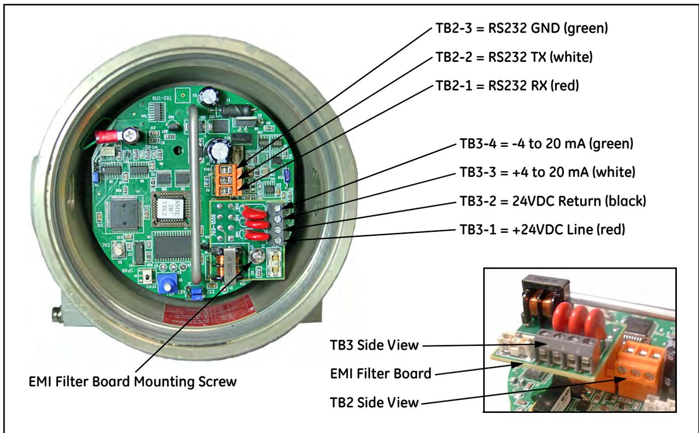
Figure 88: XMTC with EMI Filter Board - Wiring Connections
