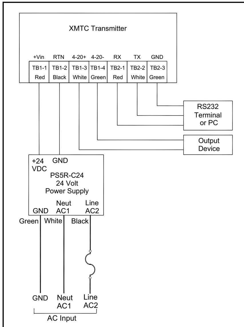
Figure 9: Interconnection Diagram
