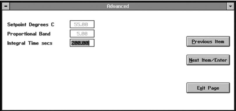
Figure 77: Integral Time secs in the Heater Window
