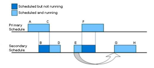
At point A, the primary schedule starts its job. At point B, the secondary schedule should start its job, but is preempted by the primary schedule's job, which is still running. At point C, the primary job is done, either by completing the defragmentation, or by having its allotted time elapse. At this point, the secondary schedule's job can start, so it does. The secondary job continues until its originally scheduled time slot is up, or the engine completes, whichever is first.
