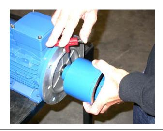
26) Pull out the magnet from motor shaft using an extractor
