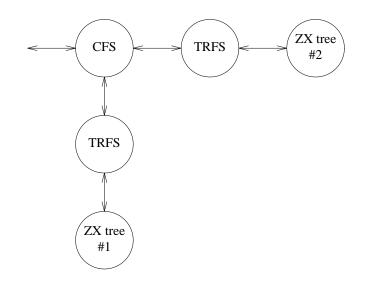
Figure 4: Tracing calls to the cache and the cached trees in CFS using a file server stack.
