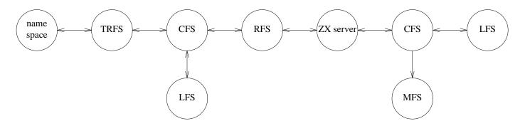
**Figure 3:** *Full fledged ZX file system stack using many file servers for caching and tracing.* CFS accepts ZX calls and relies on *two* ZX trees to serve them. It assumes the first one is a lot more cheaper than the second one, and uses the former as a cache of the latter. But, the two ZX trees used by CFS can be anyone.
