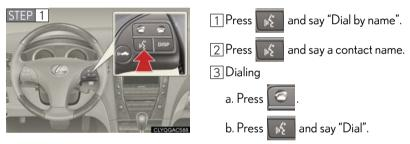
Pressing this switch turns the voice command system on. Say a command after the beep.
