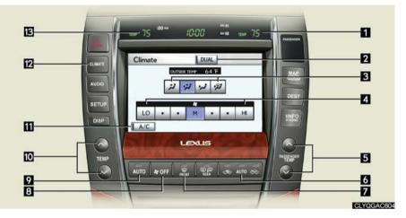
8 "OFF" button 1 Passenger side temperature display 2 Dual mode button 9 Automatic mode button 3 Air outlet display 10 Driver side temperature control 4 Fan speed display 11 Cooling and dehumidification function on/off button **5** Passenger side temperature control Air conditioning operation screen 6 Outside air/recirculated air mode display button button **13** Driver side temperature display 7 Windshield defogger
