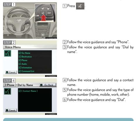
: Pressing this switch turns the voice command system on. Say a command after the beep.
