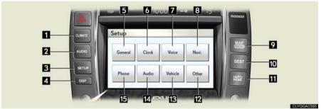
Press the button to display the screen. The "Setup" screen shown in the above illustration is displayed when the "SET UP" button is pressed.
