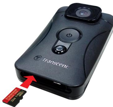
1. Insert a microSD memory card into the card slot on the bottom of the camera.
