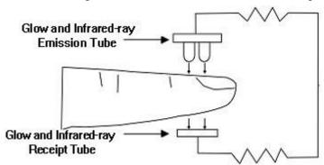
Figure 1. Operating Principle
