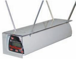
Competition Electronics offers an optional Debris Shield which can help to protect your chronograph from flying debris and paint. However, we offer no guarantee that it will protect your chronograph from damage. This item is shipped with a protective film to be removed before use.
