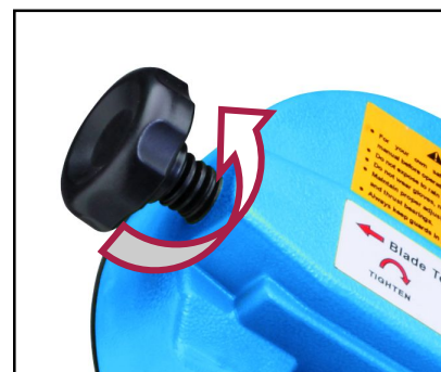
Figure 17 - Blade tension reduction.
