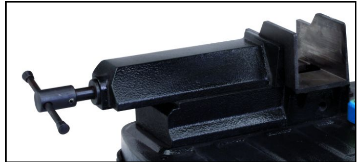
Figure 7 – Vice adjustment screw.
