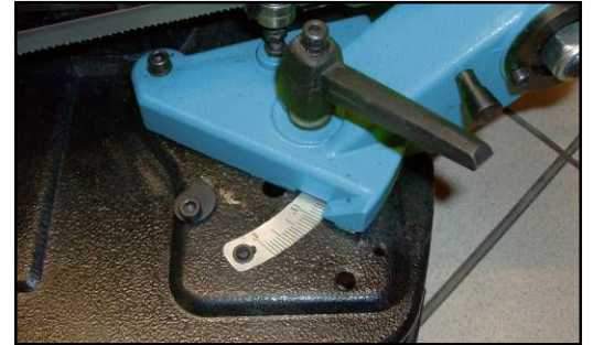
Figure 13 – Adjusting the head position.
