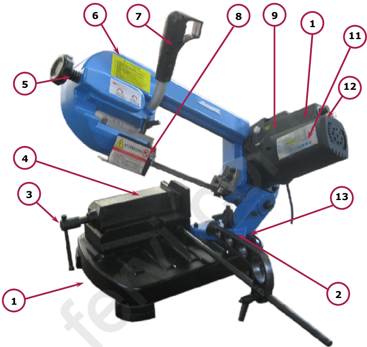
Figure 2 – Close-up of the main parts of the saw.
