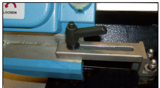
Figure 9 - Blade cover locking lever.
