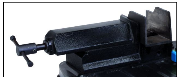
Figure 14 – Adjustment and locking of the vice.
