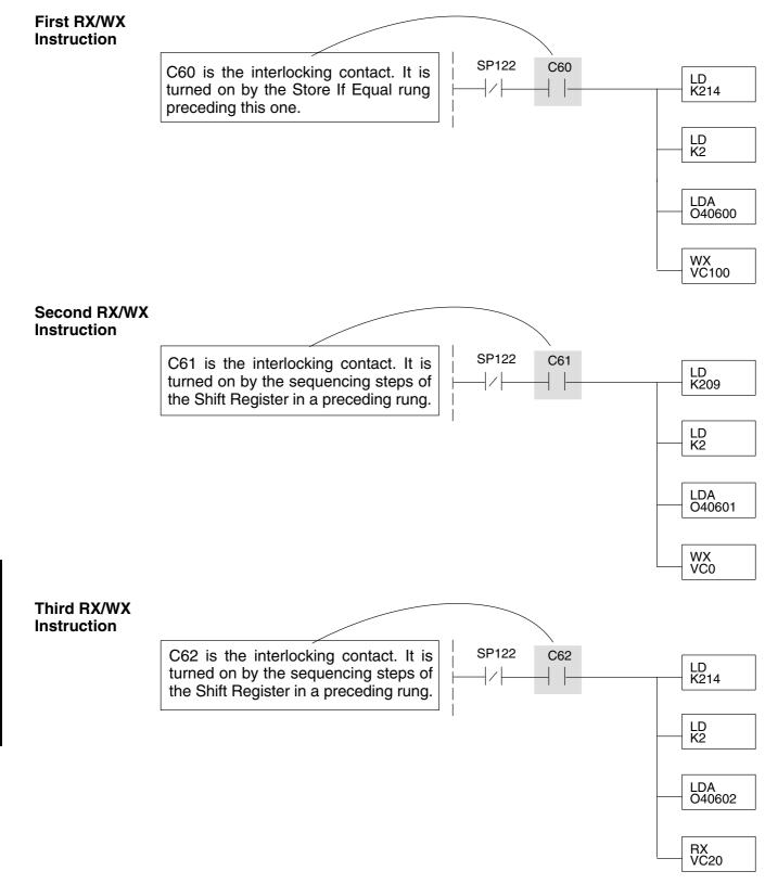
After this rung is executed, the Shift Register shifts the high bit from C62 to C63 on the next CPU scan. C63 resets the Shift Register to zeros, the Store If Equal sets the C60 bit, and the CPU executes the first RX/WX instruction.
