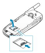
4. Insert the SIM card, ensuring that the cut corner faces top left and the gold contacts of the card face into the phone.
