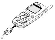
2. Connect the adapter to a standard AC wall outlet.
