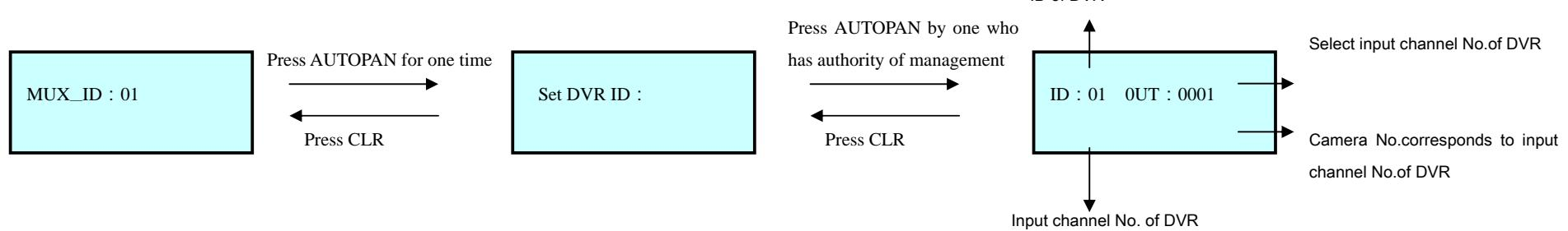
3. Under the state of Multiplexer, press AUX to display the Multiplexer's ID of protocol and baud rate of communication.
