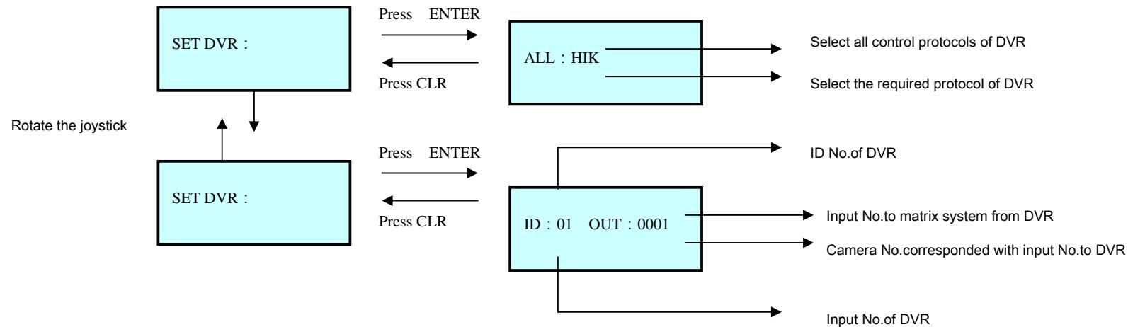
**Note: Rotate the joystick to select the required protocol and input address No by digit-key. After selection of the protocol, press ENTER to make acknowledgement or press CLR to exit the setting.**
