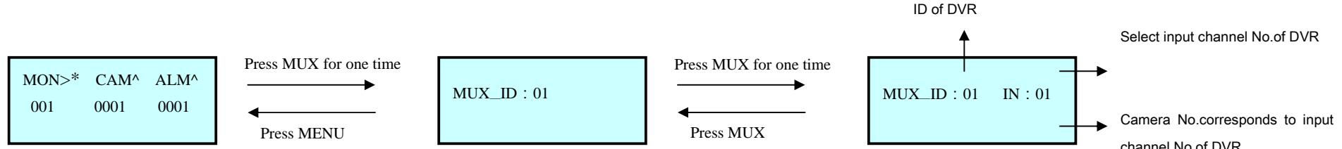
2. Under the state of Multiplexer, press NEXT to select ID of the current Multiplexer. One who has authority of management can setup input channel No.of Multiplexer corresponding to camera No.
