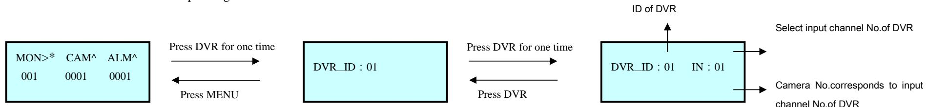
2. Under the state of DVR, press NEXT to select ID of the current DVR. One who has authority of management can setup input channel No.of DVR corresponding to camera No. (Setting is also available in main menu.)
