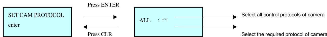
Rotate the joystick to select the required protocol and input address No by digit-key. After selection of the protocol, press ENTER to make acknowledgement or press CLR to exit the setting.
