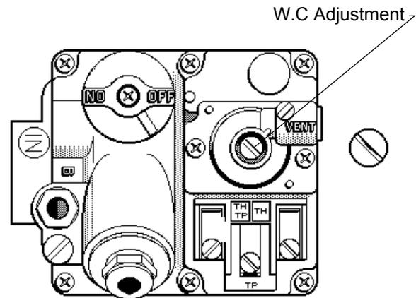
HONEYWELL VALVE MV & IID W. C. Adjustment
