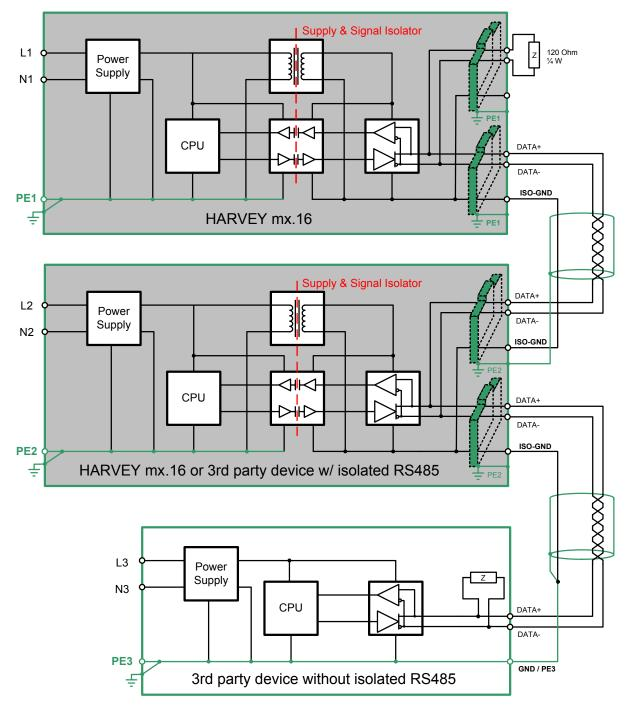
Internally the RS-485 circuit is carried out isolated with regard to signals and power supply. This structure avoids ground loops which may occur in systems with long distances between the protective earth (PE) -grounding points and which may lead to communication faults. Each RS-485 interface of HARVEY mx.16 offers a ground signal which is isolated from PE-ground. Only the RJ45-shield is connected to the PE-grounded device housing.
