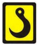
generating set by attaching to the engine or alternator lifting lugs, lifting points on the base frame or canopy.
