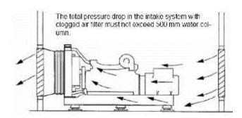
Users can use metal plate or canvas to make a wind guide cover, the connection between wind guide cover and the radiator shall be soft connection, so that to cut off the transmission of vibration from the generator set, and also ensure the hot air exhaust to outside thoroughly.
