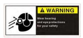
! Generating sets that are not equipped with sound attenuating enclosures can produce noise levels in excess of 105 dB (A). Prolonged exposure to noise levels above 85 dB (A) is hazardous to hearing.
