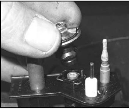
Figure 6.6 Pull off pilot hood and set it aside. NOTE: Do not remove the retaining clip from the hood.
