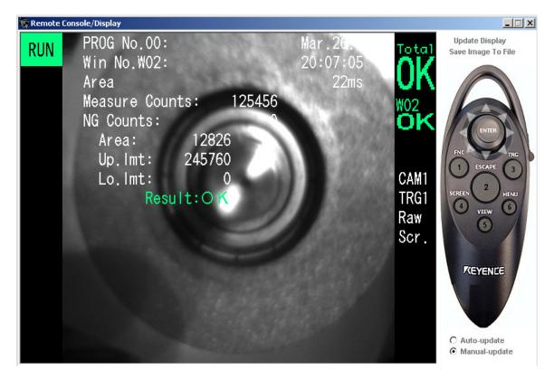
The Remote Console/Display window allows the user a graphical remote interface to the CV-2100. The left hand area of this window is used to display a BMP image representing the current CV-2100 display. The right hand area of this window contains a pseudo-remote console (A.K.A. pendent) along with some options and command links.
